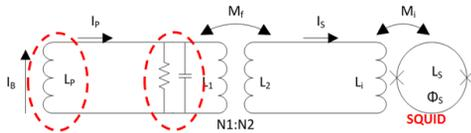
Figure 2: Coupling circuit that converts the beam current into a magnetic flux to be measured by the SQUID.
