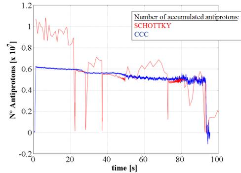
Figure 8: Comparison of the “intensity” (number of antiprotons) measurement between the longitudinal-Schottky and the CCC monitors, during one AD cycle (with 10% of nominal intensity).
