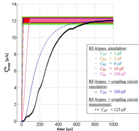
Figure 6: Simulation of the signal (referred to equivalent beam current) coupled to the SQUID at AD beam injection, considering the RF-bypass alone and also the combined effect with the coupling circuit filter. And laboratory measurement using a signal generator passing a similar current signal through a beam simulating wire.
