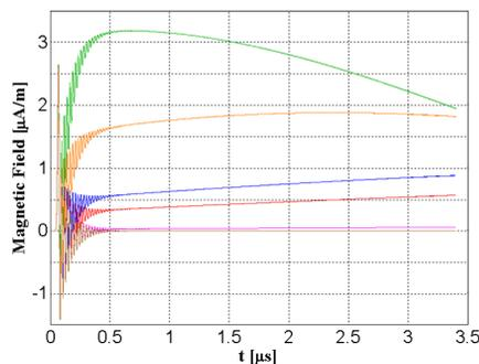
Figure 5: Time domain simulation of the magnetic field coupled to pickup core, induced by the passage of a single bunch of the AD injection beam.
