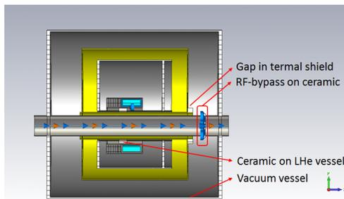
Figure 4: Simplified model of the real cryostat used in time-domain simulation of a single bunch. The CCC shield is shown, but was not considered for the simulation.
