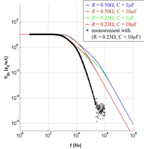
Figure 3: Theoretical frequency response of the coupling circuit alone, for various values of R and C. And laboratory measurement of the frequency response of the complete system (coupling circuit plus cryostat) using a beam simulating wire passing through the cryostat beam pipe (in black).
