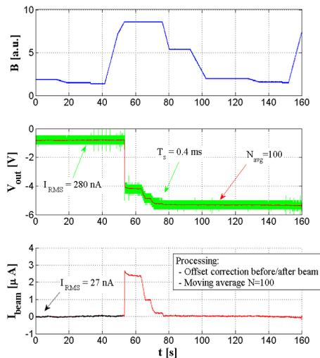
Figure 7: Top Plot: Magnetic Cycle of AD Dipoles in arbitrary Units. Middle plot: SQUID/FLL raw signal of beam current (in green), and same signal filtered with a moving average (in red). Bottom plot: calibrated beam current measurement after filtering and baseline recovery (before beam injection and after extraction).
