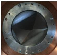
Figure 4: Picture of the newly third skimmer with sizes  $4.0 \times 0.4$  mm<sup>2</sup>.
