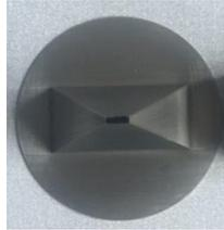
Figure 2: Picture of the previously used third skimmer with sizes  $7.2 \times 1.8$  mm<sup>2</sup>.
