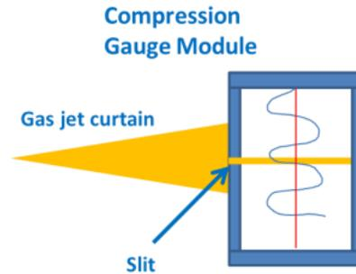
Figure 6: The schematic of the compression ion gauge module.
