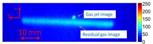
Figure 5: Images of the electron beam from both gas jet (smaller size third skimmer) and residual gas.
