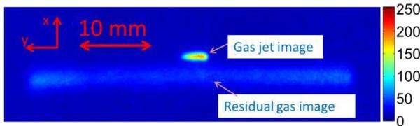
Figure 3: Images of the electron beam from both gas jet (larger size third skimmer) and residual gas.
