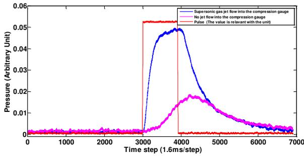
Figure 7: Measured pressure change of the moveable ion gauge.
