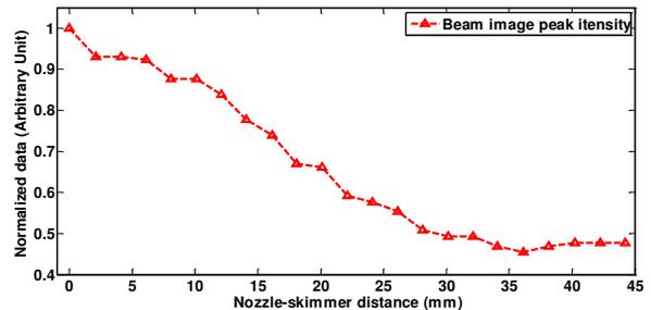
Figure 11: Plot of Peak intensity of the image from gas jet versus the nozzle to first skimmer distance.
