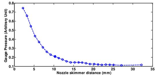
Figure 10: Plot of sampled supersonic jet pressure measured at the first dump chamber by the moveable gauge module versus nozzle to first skimmer distance.
