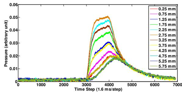
Figure 8: A vertical pressure scan of the gas jet from the moveable gauge module. Plots show the pressure curve at a few selected gauge positions.
