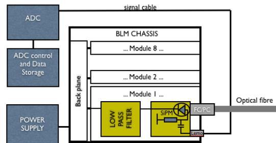
Figure 2: Schematic view of the oBLM read out.
