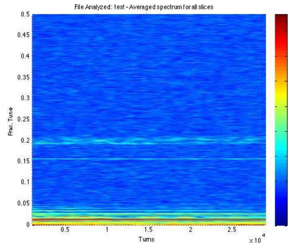
Figure 10: Closed-Loop (feedback on) spectrogram of Figure 7 transient. The beam is unstable in these conditions, Q26 lattice,  $\nu_y = 0.185 \nu_s = 0.006$ . A small amount of motion at mode zero is seen, this driven motion is reduced by the feedback gain. The feedback control keeps the mode 1 and 2 sidebands at the noise floor of the feedback receiver, or roughly 6 microns.
