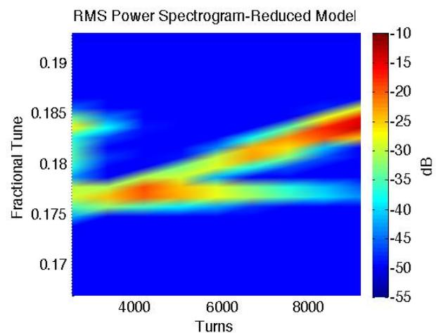
Figure 6: Beam motion spectrogram response for the reduced beam model (same excitation as Figure 1). Comparing with the physical measurement we see very close agreement between the oscillation frequencies and the amplitudes of the excited motion.
