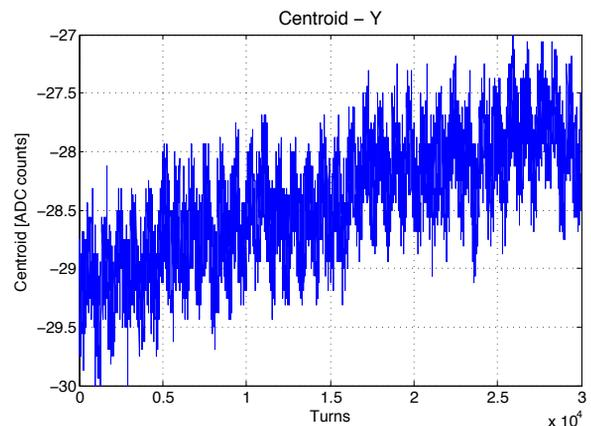
Figure 9: Closed-Loop (feedback on) time-domain recording of bunch motion, bunch samples averaged to show the vertical centroid. The same beam conditions as Figure 7 (mode 0 instability) but motion is controlled by the feedback system. Vertical sensitivity is roughly 14  $\mu\text{m}/\text{count}$ .
