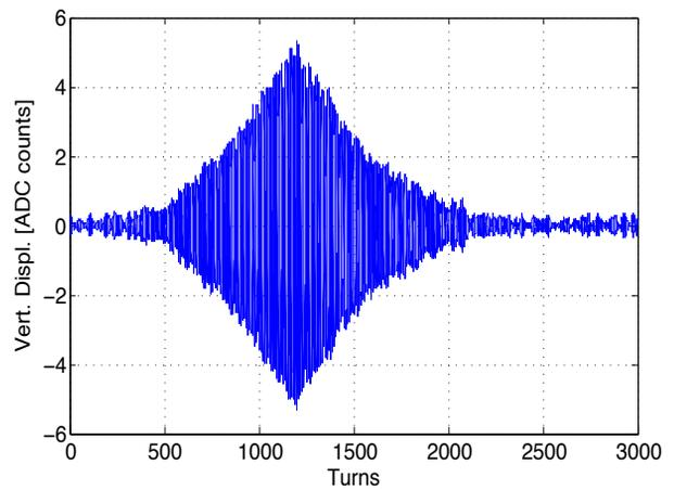
Figure 11: Time domain grow-damp study, SPS beam with excitation of mode 0, followed by damping through the feedback system with gain x4
