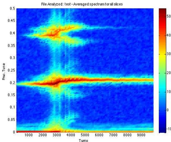
Figure 8: Open-Loop (no feedback) spectrogram of same transient as Figure 7. The beam is unstable in these conditions,  $\nu_y = 0.185 \nu_s = 0.006$ . At turn 2000 chromatic effects show sidebands of the mode zero motion, and with charge loss these end at turn 4500. Significant intensity-dependent tune shifts are seen as charge is lost in the transient.
