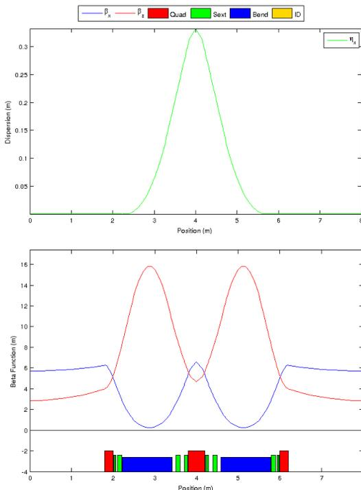
Figure 1: The optical functions for single DBA cell.
